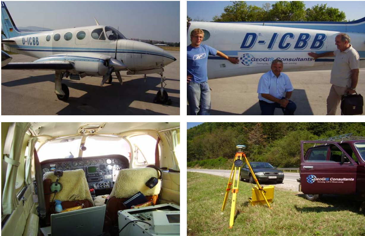
Picture 1. Laser scanning of the corridor from the Town of Leskovac to FYRM border, 2007 (Aircraft with integrated GPS, INS and laser scanner and GPS transmitter on the terrain)
