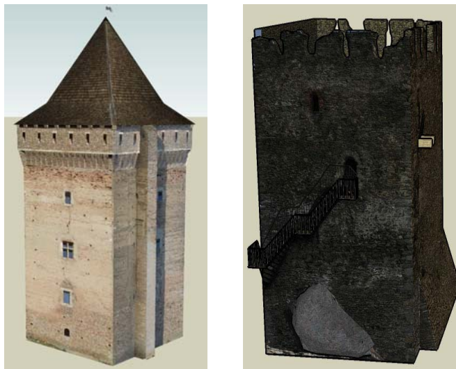
Picture 6. 3D model of the culturally significant buildings based on data from laser scanning and digital photographs of high resolution (The Tower in Bac and the Tower in Vrsac, GeoGIS Consultants 2008)
