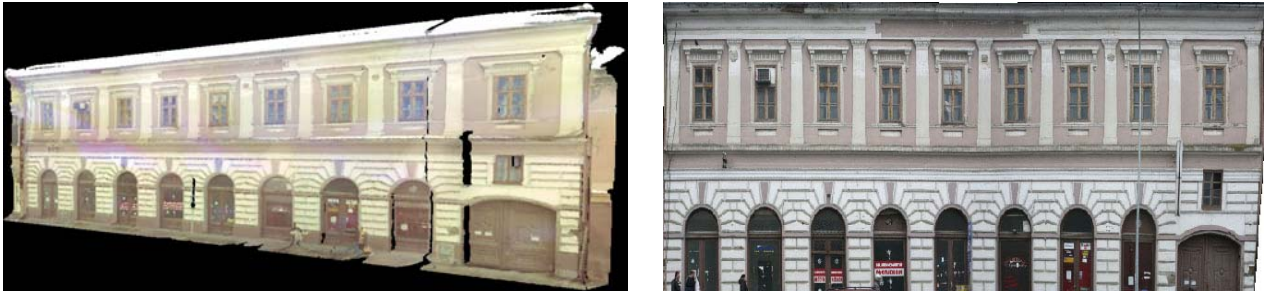
Picture 5. Laser scanning of the building façade in Vrsac, ortho-photo plan of the part of the façade
